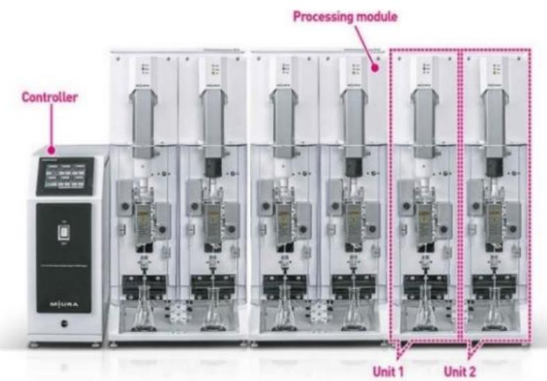
A Miura GO-6HT for the purification of samples for dioxin, PCB, PBDE and PCN analysis above and a chromatogram of tri- till hepta-PCB on the right
